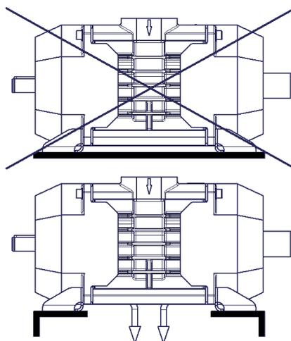
Fig. 4: Installation position
