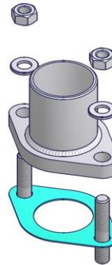
Fig. 5: Assembly example for suction flange
