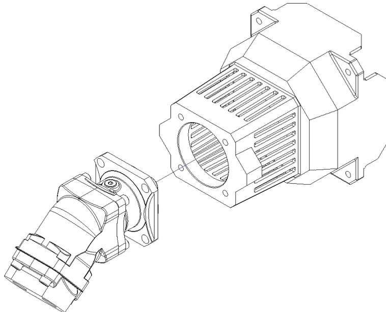
Fig. 8: Installing the hydraulic motor
