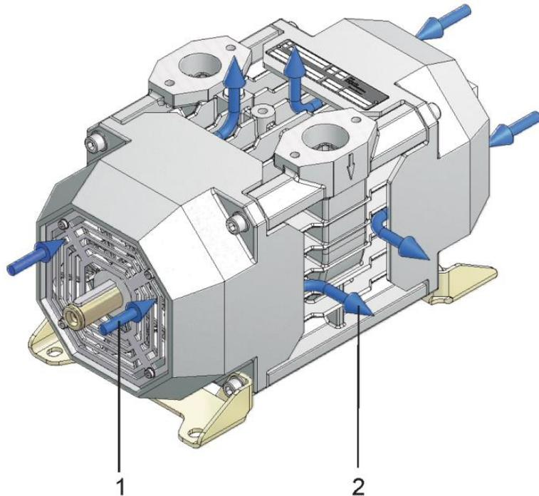
Fig. 6: Cooling air guide
