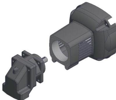
Abb. 8: Montage Hydromotor
